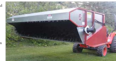
Figure 1. A loader-mounted brush stripper can be an effective way to harvest NWSG seed. Photo courtesy of Tannas Environmental Services.
